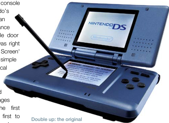
Double up: the original DS featured two ARM CPUs, two displays and two game slots – one for Game Boy Advance cartridges, the other for Nintendo's new flash cards.
